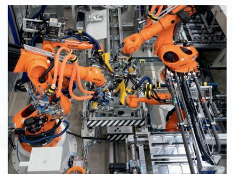
Assembly and fixing of the battery modules
