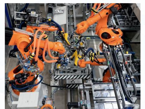
Assembly and fixing of the battery modules
