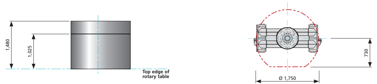
Basic machine with max. interference range with/without optional pallet changer with displacement axis
