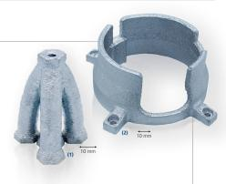
$^{(0)}$ 180 Hz printing frequency; 590  $\mu$ m drop diameter; 115 min print time  $^{(0)}$ 150 Hz printing frequency; 685  $\mu$ m drop diameter; 160 min print time
