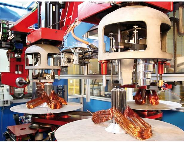
WINDING/INSERTING MACHINE E200 WIZE
