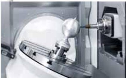
spindles that run at 15,000 rpm, but can go as high as 18,000 rpm. The machines typically travel at 2,560, 1,650 and 3,540 ipm in the X, Y and Z axes respectively.
